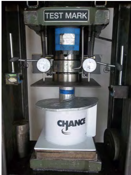
FIG. C-1 - P3 HELIX STRENGTH SET-UP
