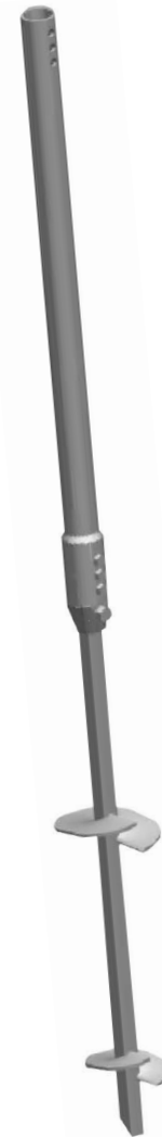
PILE ASSEMBLY WITH TRANSITION COUPLER FIGURE 7-46
