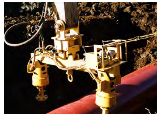
DIFFERENTIAL PRESSURE TORQUE INDICATOR FIGURE 6-15
