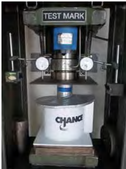
Fig. C-1 – P3 Helix Strength Set-Up
