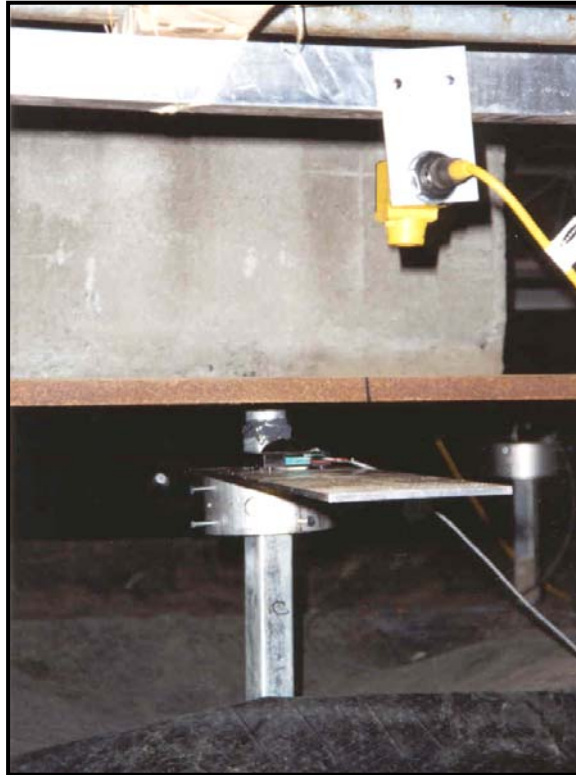
Figure 3.17 Support System for OMNI-BEAM™
