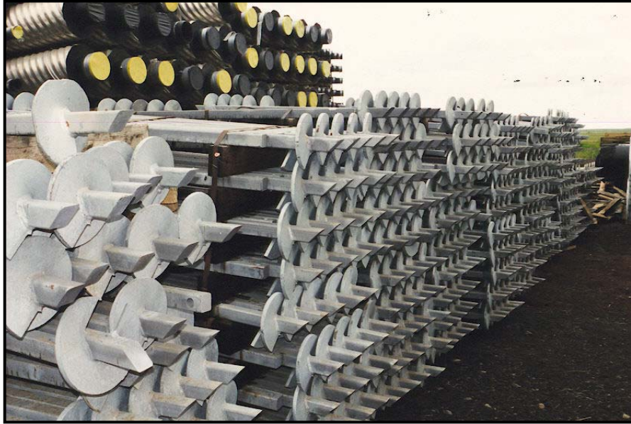
Figure 1.5 Helical Pier Stockpile in St. Michael, Alaska
