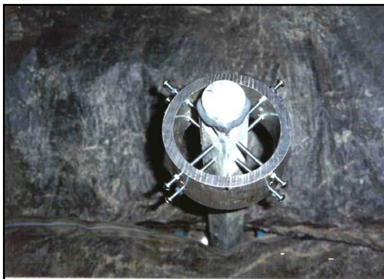
Figure 3.18 Aluminum Collar Bolted to Sides of Pier to Support Arm for Settlement Measurements
