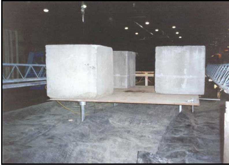
Figure 3.25 Loading Piers with Three Concrete Blocks (view looking North)
