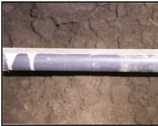
a. Milled Rod with Potting Compound
